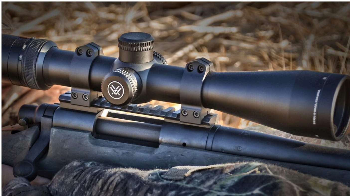
Figure 2. A bolt-action rifle with a scope mounted on a Warne M673M tactical Picatinny rail.
